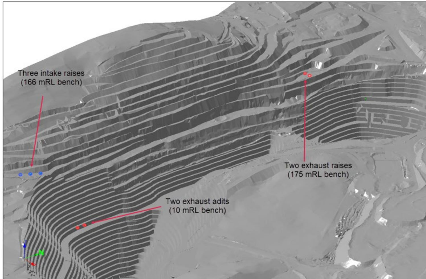
Figure 24-15: Vertical Development Items with a Surface Expression in Vicinity of the Open Pit
